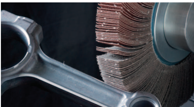
PRODUCT: 8"x 1"x 3" 120 grit Flap Wheel APPLICATION: Deburring automotive part.
