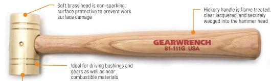
Striking face is machined flat for even blow distribution
