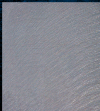
Properly finished stainless steel plate.
